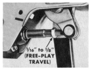
fective solid pedal of ½ to ¾ of the total pedal travel is considered satisfactory. But the brake *pedal free-play* travel should be ½ to ½. You can get this by lengthening or shortening the master cylinder push rod. This will provide the correct clearance of .015" to .030" between the push rod and piston.
