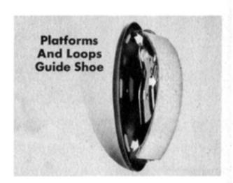
The big basic change involves the dust shield and brake shoes. Three platforms, pressed in the shields, and three loops formed on the sides of the shoes are key factors in operation. The loops guide the shoe on the platforms, and keep it in accurate alignment with the contact surface of the drum.
