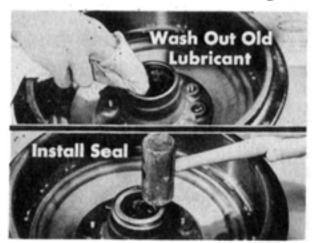
the old lubricant. Always remove the cone and roller assemblies and seals, and wash the old lubricant out of the hub. Wash the bearing, and then repack them with new lubricant. Add 13/4 oz. of lubricant to the inside of the hub. Install the bearings and the new inner seal.
