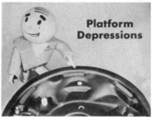
**Shoes.** You will immediately notice points of difference between the brake shoe of the 3-platform brake and the shoe from the former-type brake. Holes for the two dampener coil spring rods are closer to the center of the web, for one point. Instead of the *single* contact loop at the edge, the new shoes have *three* contact loops . . . and each loop is much shallower in design.
